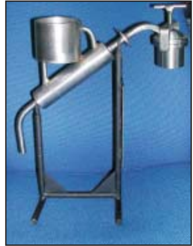
Accessible technologies to separate mercury from gold in a safe manner, such as this UNIDO retort, need to be promoted.
