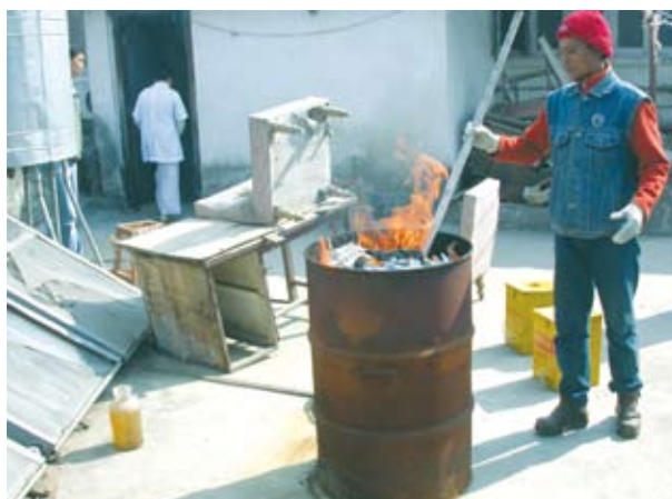
Burning waste in a drum incinerator on the rooftop of a hospital, Nepal (Photo: WHO)
